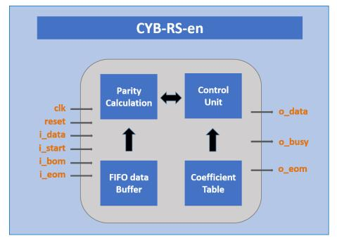
CYB-RS-en core implements the Reed Solomon encoding algorithm and is parameterized in terms of bits per symbol, maximum codeword length and maximum number of parity symbols. It is intended for use in a wide range of applications requiring forward error correction and can be targeted in any FPGA technologies.
